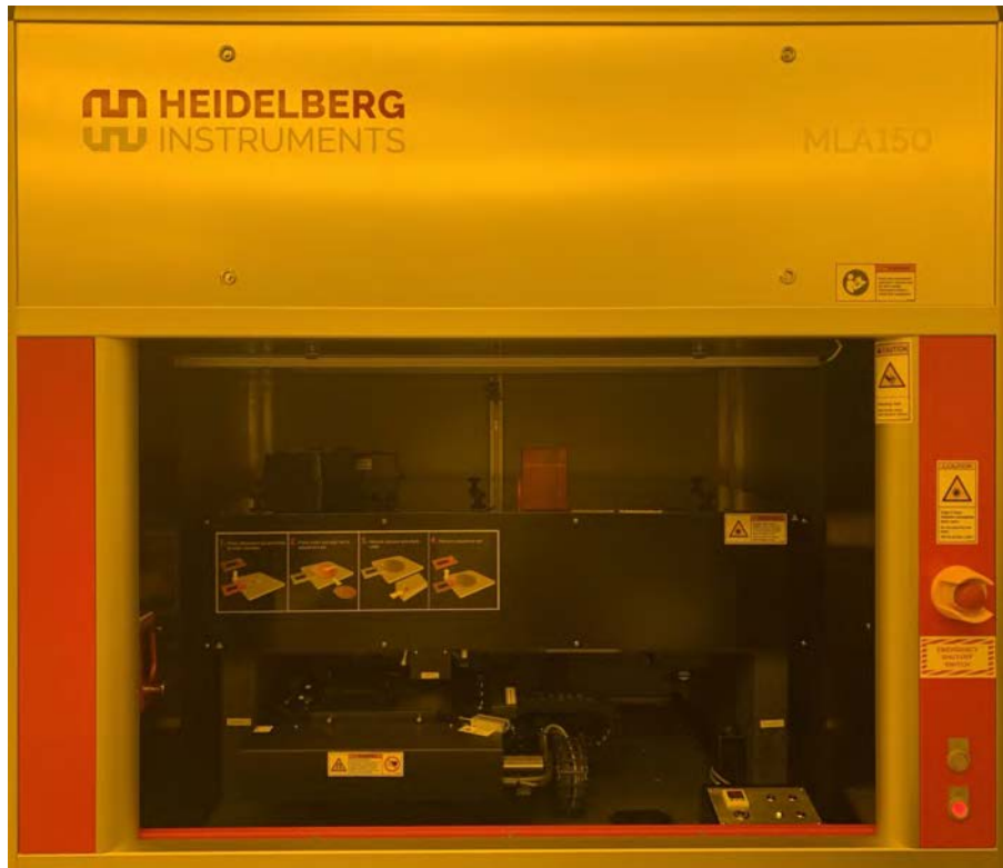
Abbildung 3.4: Photolithography MLA150 in cleanroom
