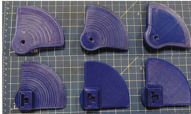
Figure 3.13: FDM printed PLA push heads. The top view is in the upper row, and the bottom view is in the lower one, on a cm grid for scale. The curvature of the top contact surface of the print heads can be identified by their print layer pattern. Left = concave, middle = convex, right = flat.
