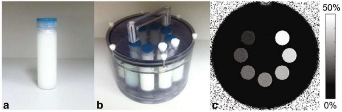
Figure 2.18: a: Photograph of a vial filled with an MR-based biomarker. b: Multiple different vials placed in a phantom holder filled with deionized water. c: The MR-based biomarker solution for each vial can be estimated using MRI. In this example, values are (beginning at the 12 o'clock position and moving counterclockwise) 0, 5, 10, 15, 20, 30, 40, and 50%.[26]
