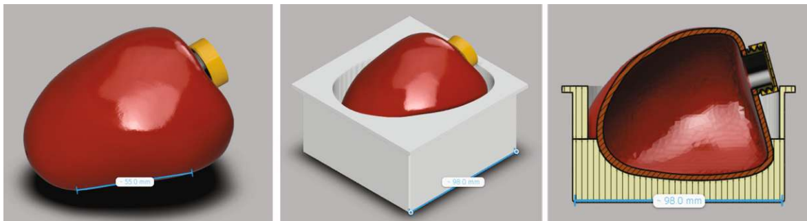
Figure 3.34: CAD render of the second iteration heart phantom with its inlay, measurement in mm for scale. Colored in red is the main heart body, yellow for the closing screw top, and gray for the heart inlay. Left: isometric view of the heart phantom. Middle: isometric view of heart phantom inside the inlay. Right: side view with a sagittal cut of the heart phantom inside the inlay.
