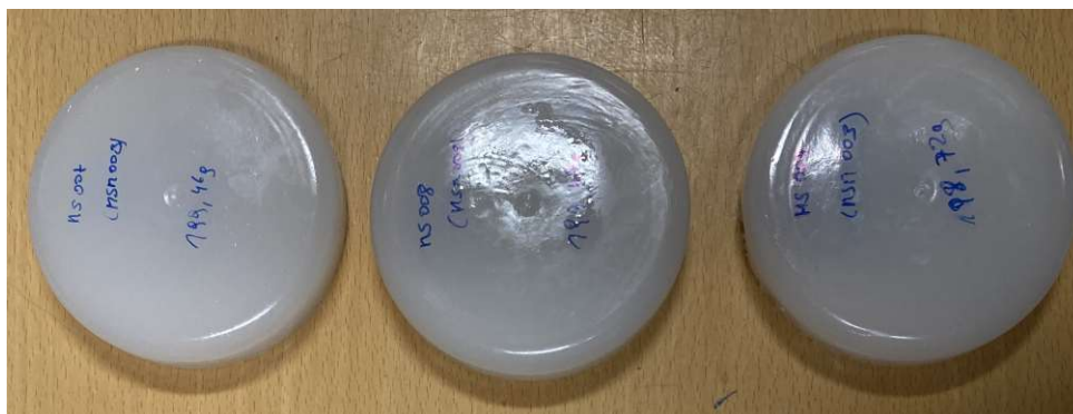
Figure 3.5: Samples MS007, MS008, MS009 (from left to right) are manufactured with micro-spheres and paraffin oil. They are moulded discs of 10cm diameter and approximately 2.2cm height.
