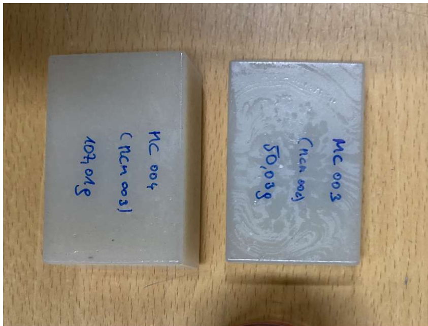
Figure 3.6: Samples MC003 and MC004 are manufactured using a mixture of micro-capsules with paraffin oil within a molding process with UV hardening in liquid resin.
