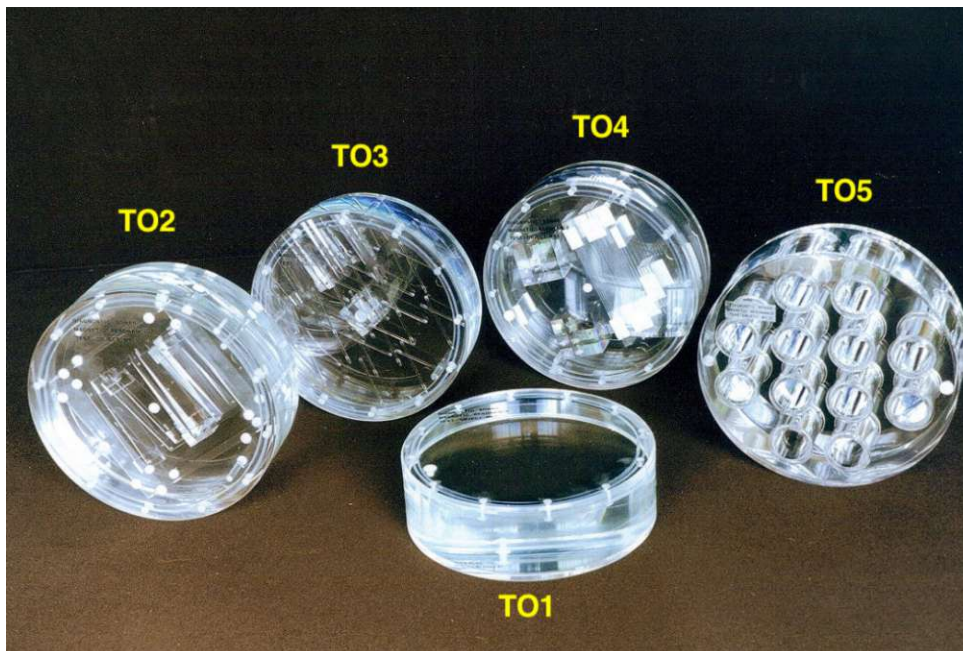
Figure 3.1: Set of the Eurospin II Test System [Elster, 2023]
