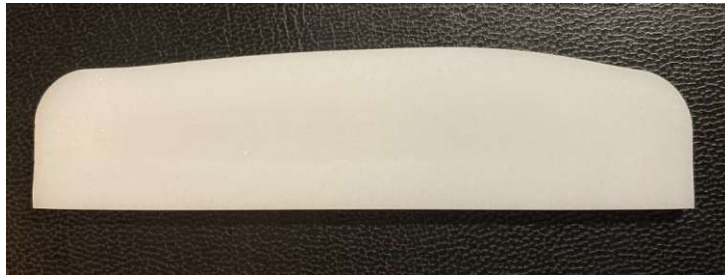
Figure 4.17: Photographic image of a slice cut in the middle of sample MS022. The inhomogeneity can also be observed in the optical transmission of the thin slices: the center being more transparent than the periphery.
