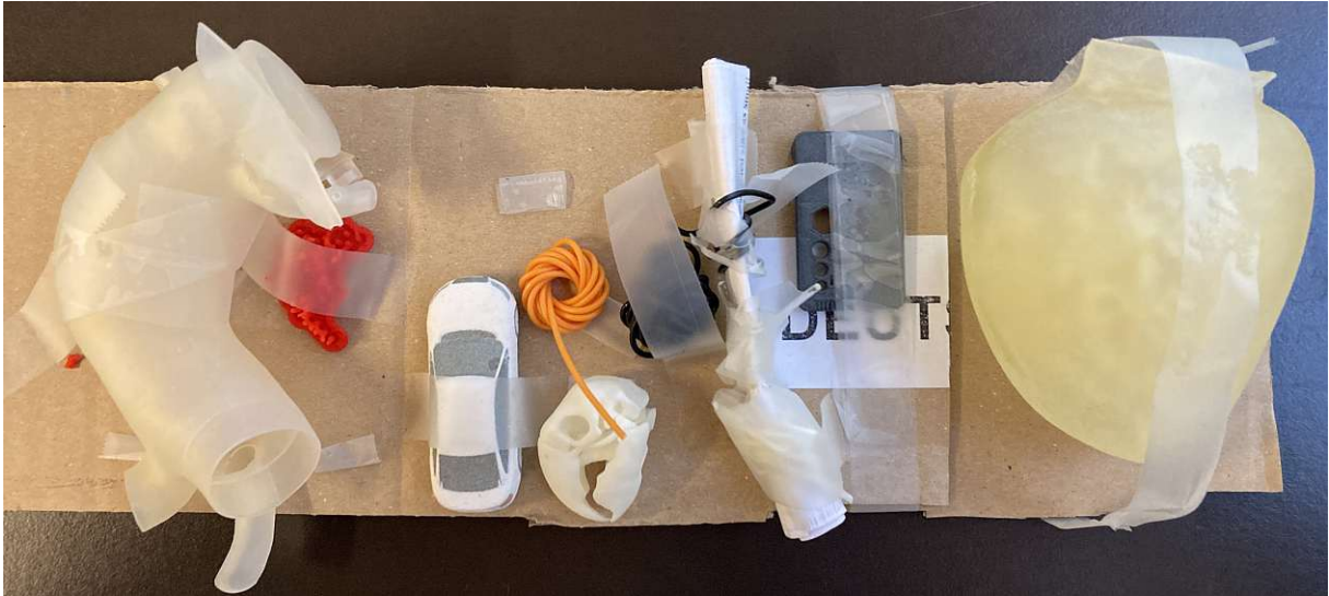
Figure 3.2: Ten samples of on site available polymers selected for MRI-visibility investigation.
