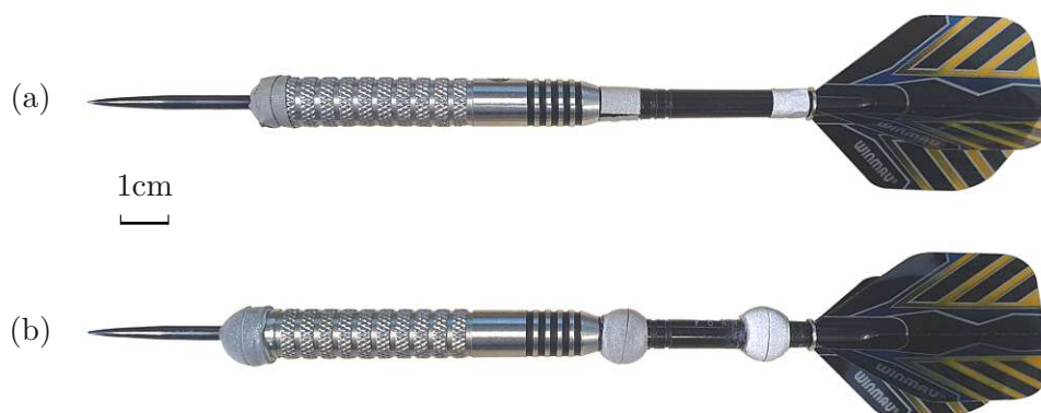
Figure 7.2: (a) Dart with reflective tape. (b) Dart with spherical reflective markers.
