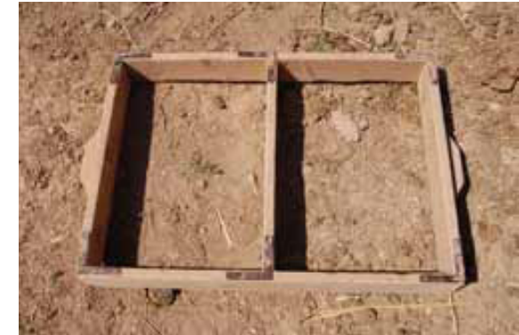
Fig.5.4. Clay bricks molds, Mecca and Dipasquale, 2009
