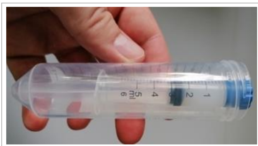
Figure 12 Preparation for PDMS centrifugation. The PDMS was centrifuged in a 50 ml falcon tube with the plunger facing downwards to avoid the formation of an air layer between plunger and PDMS ink.
