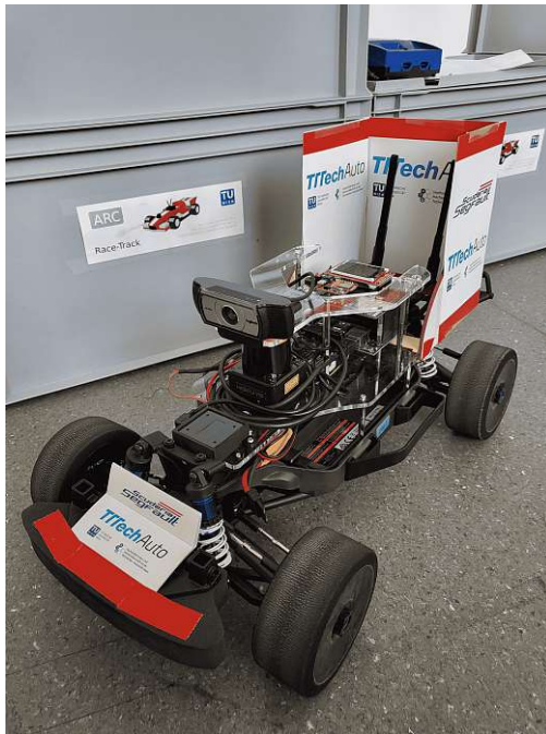
(a) F1/10-car with assembled Logitech camera.
