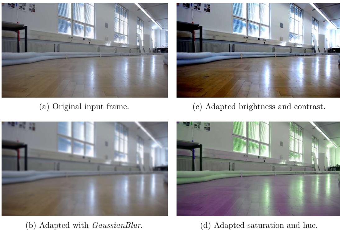
Figure 3.11: Input frames and corresponding data augmentation.
