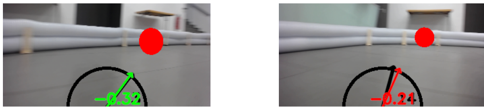
(a) Valid angle prediction within the range. (b) Invalid angle prediction with deviation from the expert.
