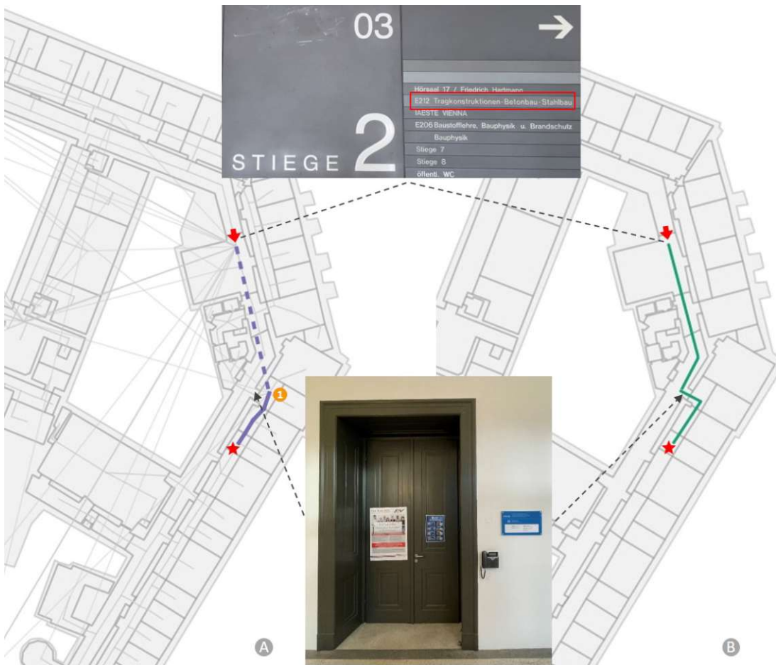
Figure 4.5 - Sample Route 2 with pictures illustrating the sign at the start and the entrance door to Department E212. (A) The resulting ISIGN route is highlighted in purple on the ISIGN graph. The semantic edge is depicted in dashed lines, while standard edges are solid. The decision point is marked in an orange circle. (B) The actual traversable route is represented in green lines on the floor plan. In both figures, the start is represented as a red arrow, with the end as a red star. The pictures are linked to their location.
