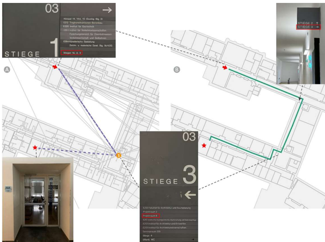
Figure 4.4 - Sample Route 1 with pictures illustrating signs en route. (A) The resulting ISIGN route is highlighted in dashed purple lines on the ISIGN graph. The decision point is marked in an orange circle. (B) The actual traversable route is represented in green lines on the floor plan. In both figures, the start is represented as a red arrow, with the end as a red star. The pictures are linked to their locations.
