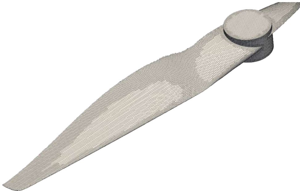
Figure 5.5: Mesh quality on the propeller surface created by using the “snappyHexMesh” tool
