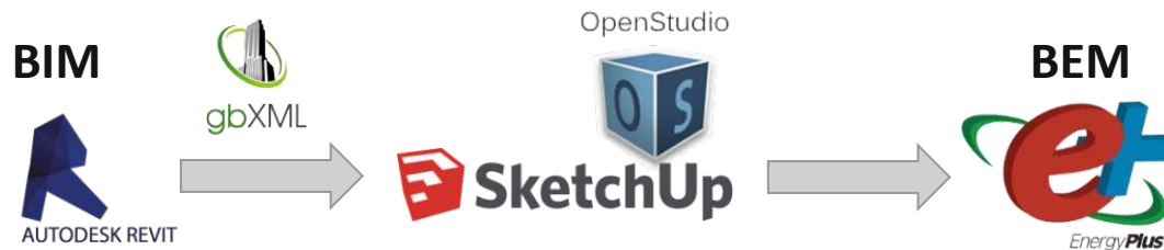
Figure 4. BIM-to-BEM workflow with state-of-the-art tools
