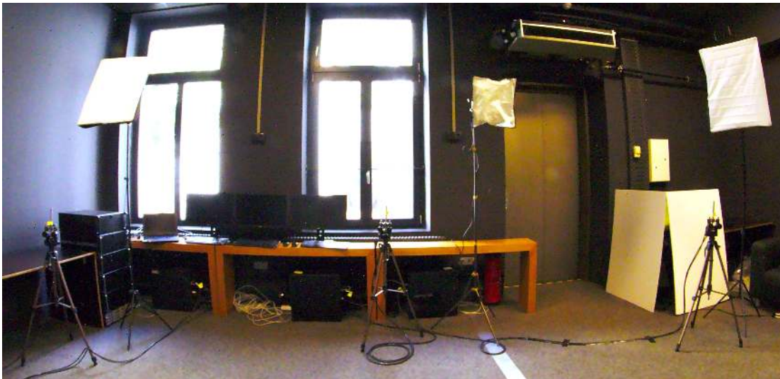
Figure 5.4: Physical system setup. The three 3DMUs were placed approximately 2 meters apart facing the scene in roughly 4 meters camera distance. Controlling and capturing PCs are shown in the back. Additional to the light provided by the windows, three studio lights with diffuser boxes were used to illuminate the captured scenes.
