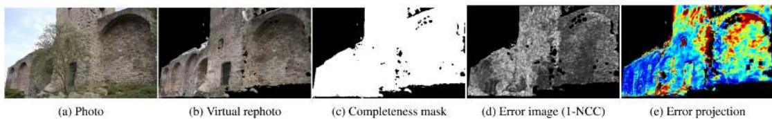
Figure 4.3: Virtual rephotography evaluation. (a) Input Image; (b) Reconstruction result rendered in the same view port as the input image. (c) A completeness mask defines the area of comparison. (d) Error Image; (e) Visualisation of error image using the jet colour map. Figure taken from [WBF + 17].
