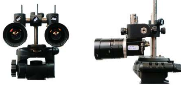
Figure 5.2: Image of a 3D Measurement Unit (3DMU). It is a stereo camera comprising two Ximea MC050CG-SY [XIM] industrial-grade cameras.
