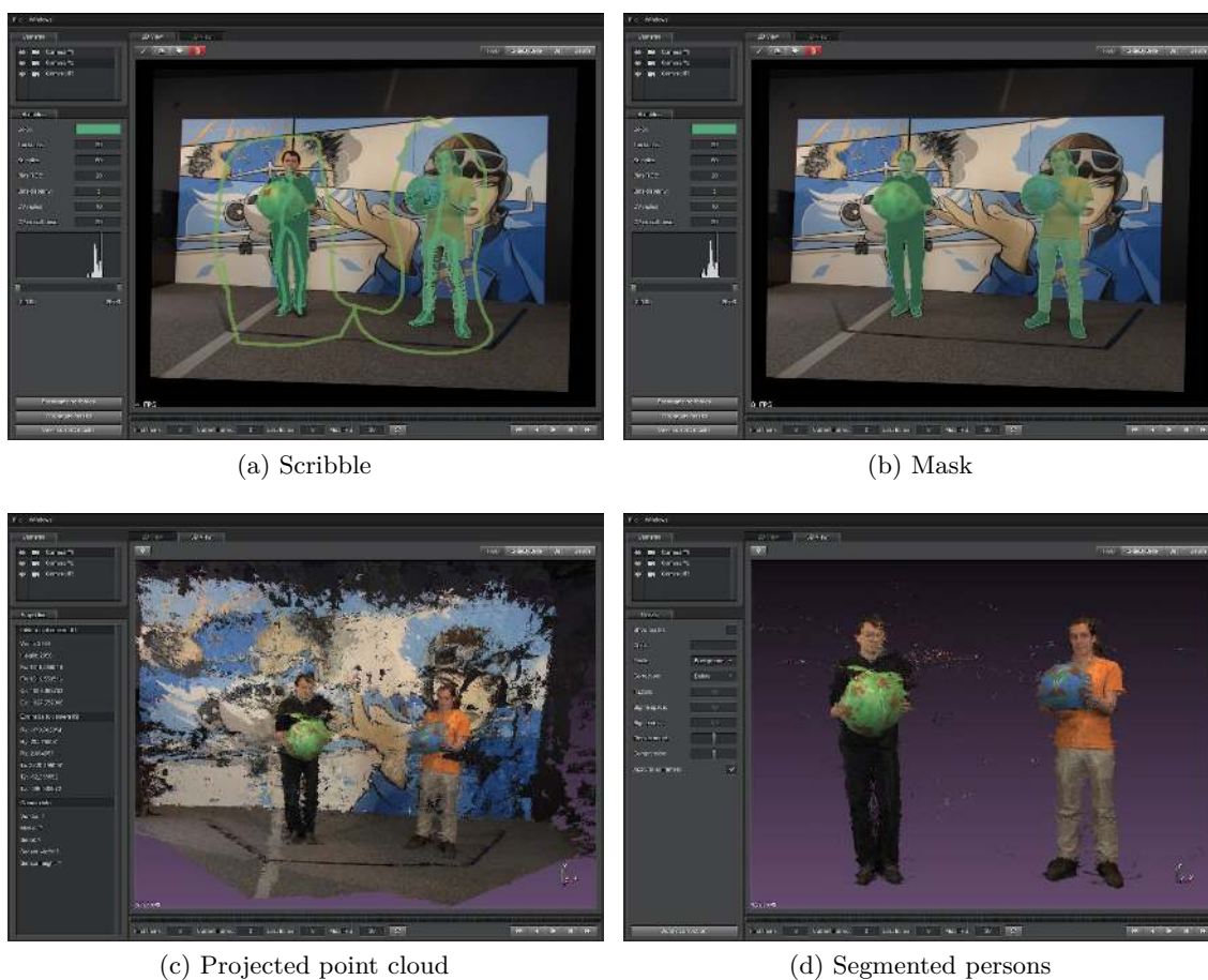
Figure 5.11: Illustration of the semi-automatic post-correction application. (a) Creation of a segmentation mask with foreground- and background-scribbles; (b) Segmentation mask obtained from scribbles in (a); (c) Full scene point cloud; (d) Segmented point cloud after applying the segmentation mask.
