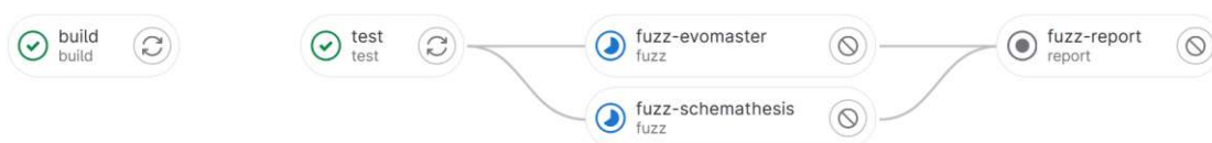
Figure 5.2: Continuous Fuzzing Basic Pipeline Jobs and Their Dependencies
