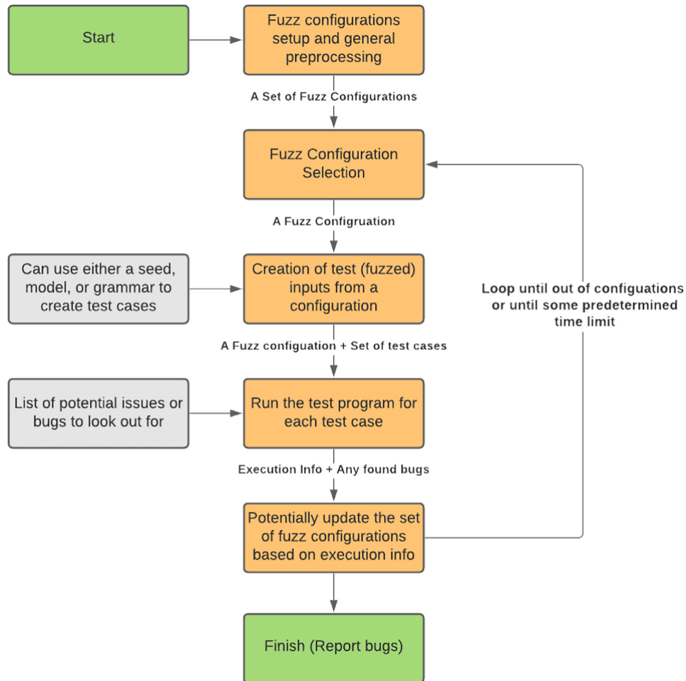
Figure 2.6: Fuzzing Algorithm Visualization [65]
