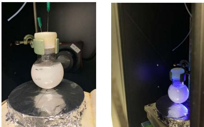
Figure 12 (left): purging of the solution, distance of sample to the lamp is 15 cm; Figure 13 (right): distribution of UV light beam on the enlarged volume.
