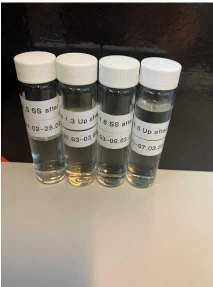
Figure 38: Sample solutions from solar simulated and upscaled experiments; respective samples (from left to right): 1/P25-Pt/He/RT/SS , 1/P25-Pt/He/RT/UP , 1/P25/He/70°C/SS , 1/P25/He/70°C/UP .
