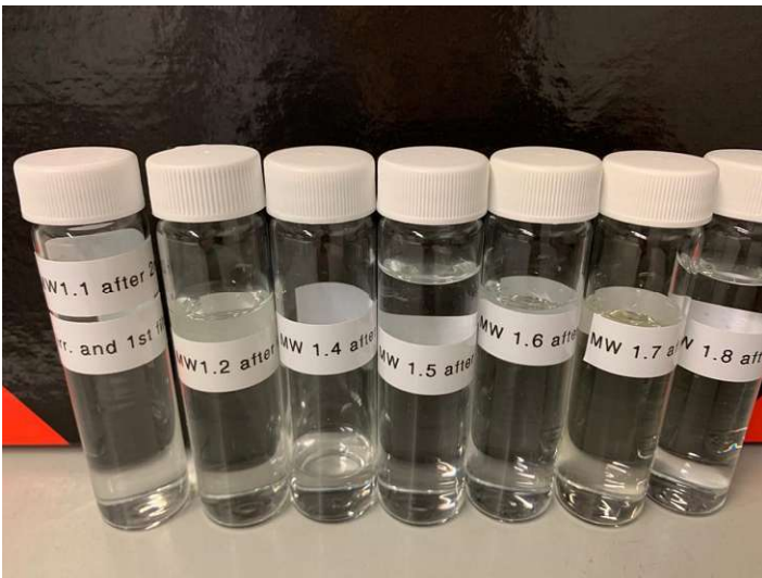
Figure 36: Sample solutions from preliminary experiments, after UV irradiation and subsequent filtration; respective samples (from left to right): 1/P25-Pt/CA/RT , 1/P25/CA/RT , 1/P25/He/RT , 1/P25-Pt/CA/70°C , 1/P25-Pt/CA/70°C , 1/P25-Pt/He/70°C and 1/P25/He/70°C .
