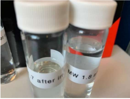
Figure 37: Comparison of sample solution colours; 1/P25-Pt/He/70°C (left) a pale yellow and 1/P25/He/70°C (right) is transparent.
