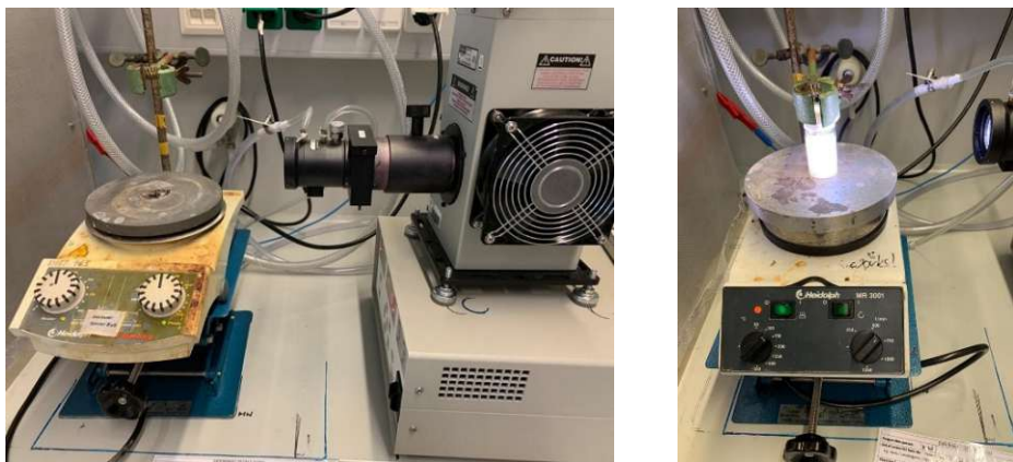
Figure 10 (left): experimental setup for the solar simulated irradiation with a Xe lamp (including an IR-filter), with a distance between sample and lamp of 15 cm; Figure 11 (right): Illumination of the sample.
