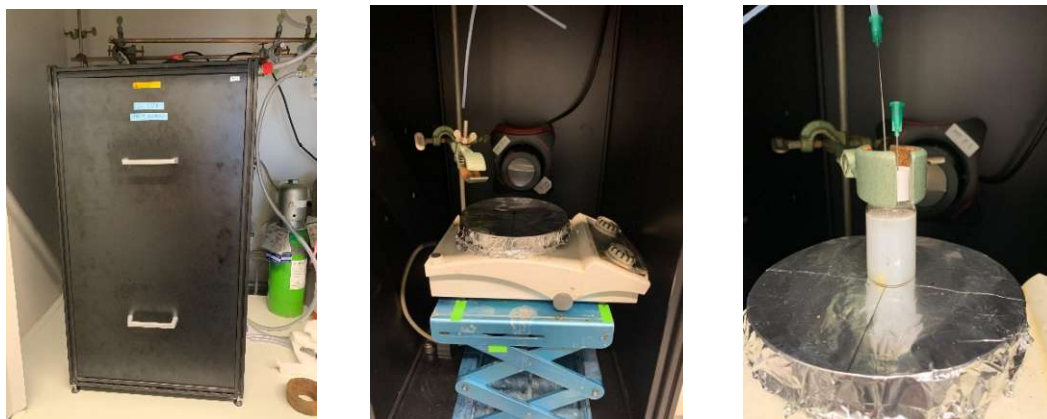
Figure 7 (left): workplace used for all experiments with a UV lamp – lovingly named Betsy; Figure 8 (middle): established setup, with markings for replicable results; Figure 9 (right): 20 mL glass vial containing sample and purging with He, distance between sample and lamp is 15 cm.
