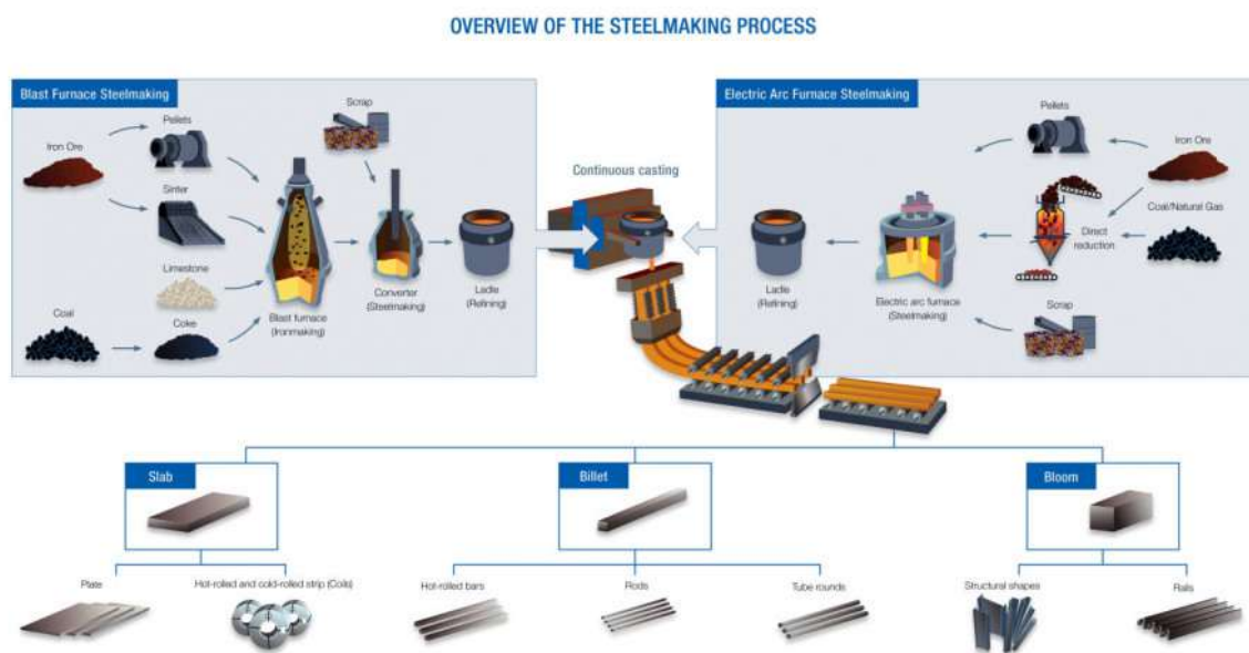
Figure 2-1 Overview of the steelmaking process [4]
