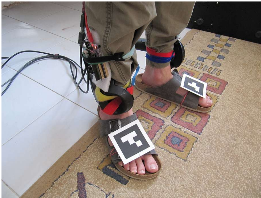
Figure 5.4: User Study Setup: The HTC Vive controller were mounted on the side of the ankles. The fiducial markers were placed near the toes. The IMU was mounted slightly above the HTC Vive controller on the right foot.
