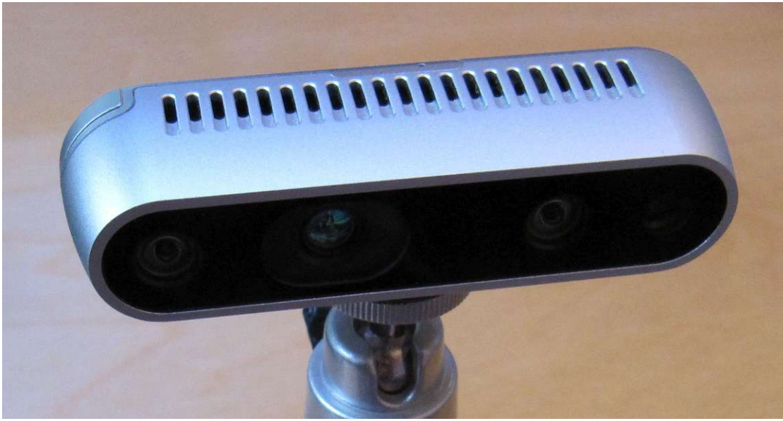
Figure 4.4: Intel Realsense Depth Camera D435
