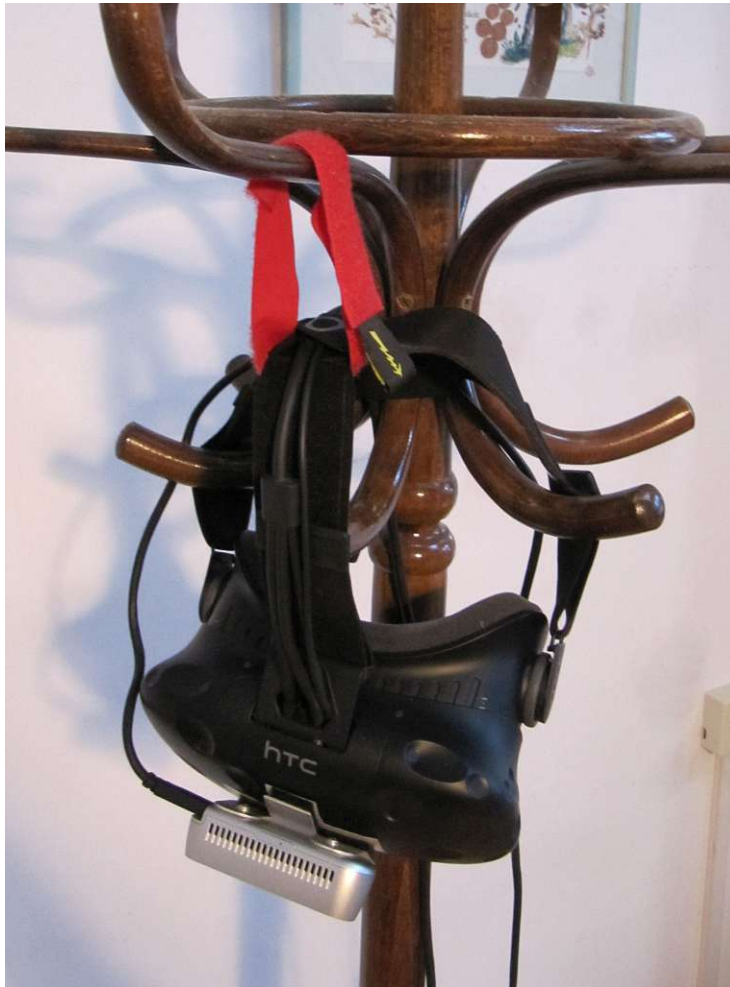
Figure 5.2: Technical Evaluation: The VR headset with the Intel Realsense Depth Camera D435 (Intel Realsense) pointed downwards to the ground
