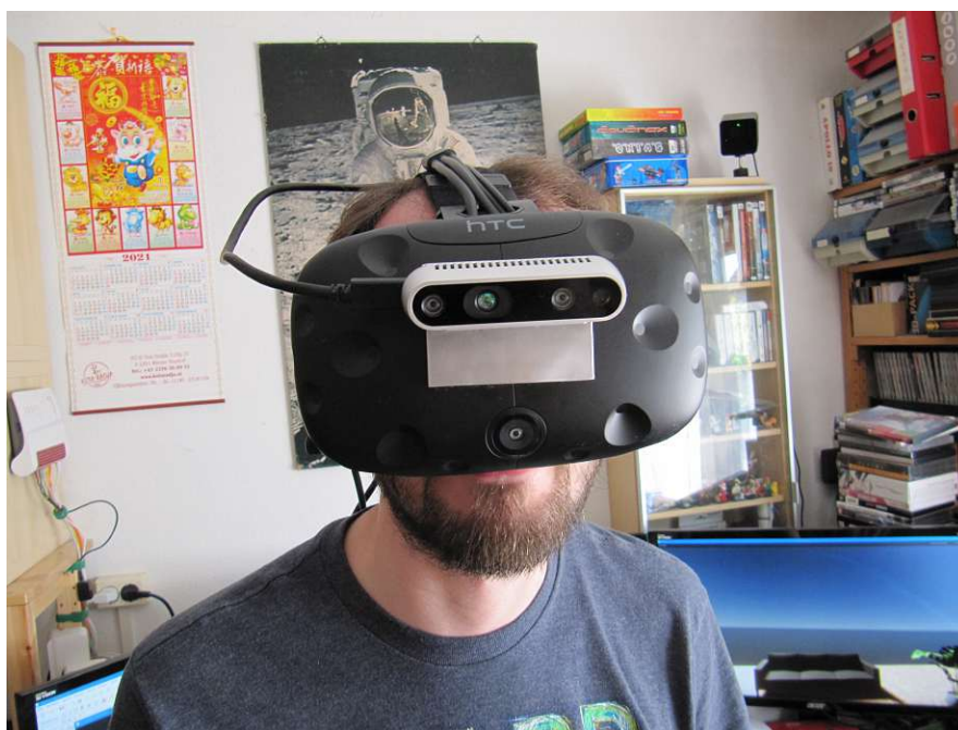
Figure 5.5: User Study Setup: The VR headset had the Intel Realsense mounted on it, placed on the front where it could not occlude the headset's sensors.
