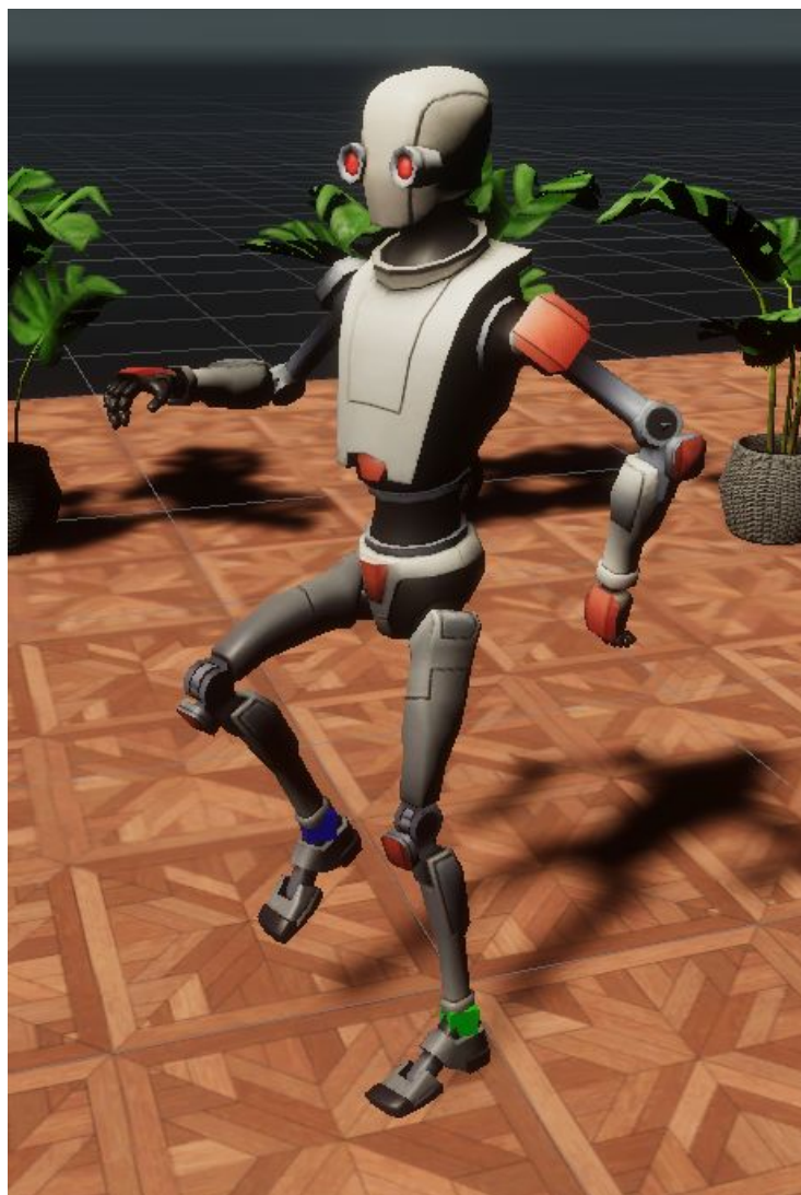
Figure 4.8: IK animation of the avatar. The green and blue cubes represent the foot positions.
