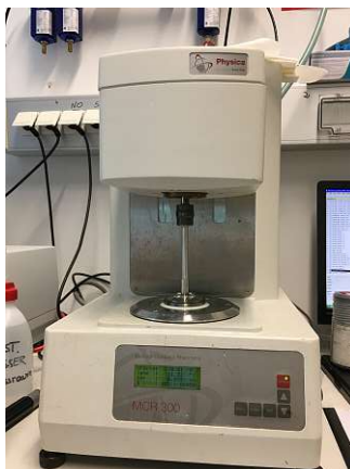
Figure 4.1: Set-up of the rheometer MCR300 by Anton Paar with a Plate-Plate measurement system
