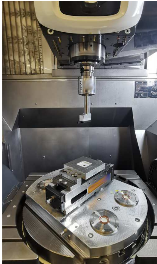
Figure 5. Prototype of roughness measurement tool in machine tool.
