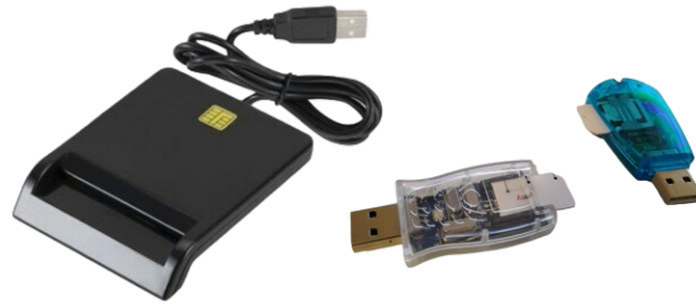
Figure 4.2: Various SIM reader devices that are supported by our SIM provider: a PC/SC reader and two different types of Serial-based SIM card reader
