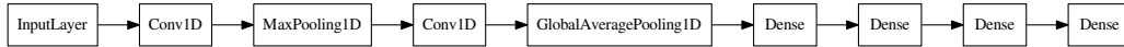
Figure 2.3: The deep network used for the classification task. Overall, the network is divided into two blocks: 1) a feature extractor (convolutional layers) that extracts a unique fingerprint from an input sequence and 2) a fully connected layers block which learns the fingerprint \rightarrow prediction mapping. The architecture is inspired from Lenet-5 [145] and adapted as a 1D-CNN.
