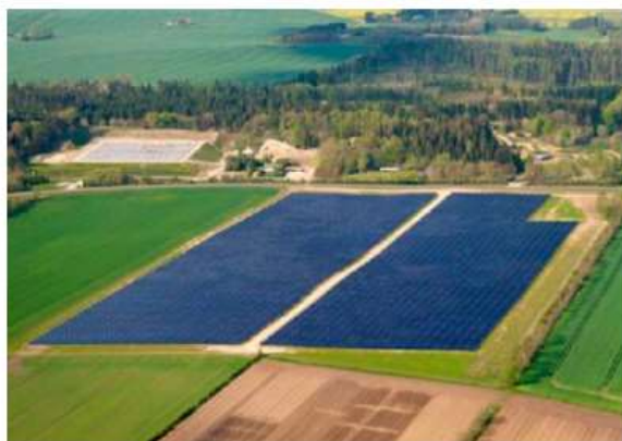
Figure 109 FPC arrays (left) and PTES (right) in Dronninglund [3]
