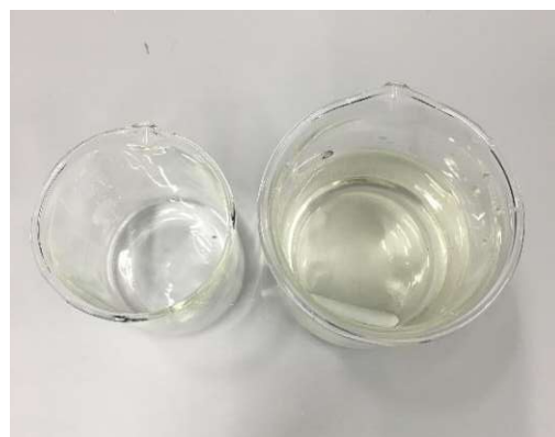
Figure 55: 0.5 M Na 2 SO 4 electrolyte (pH=6) after measuring sample shown in Figure 53 at high anodic bias (right)
