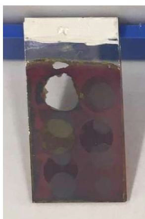
Figure 54: glass/ITO/Cu 2 O/ZnOS/NTO/Pt sample investigated at great bias of up to -1.2 V (LSV) and -0.9 V (stability test) versus Ag/AgCl
