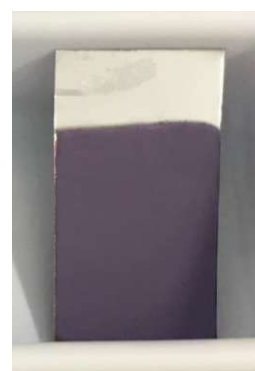
Figure 30: \text{Cu}_2\text{O} electrodeposited on stainless-steel foil at -0.50\text{ V} vs. \text{Ag}/\text{AgCl}
