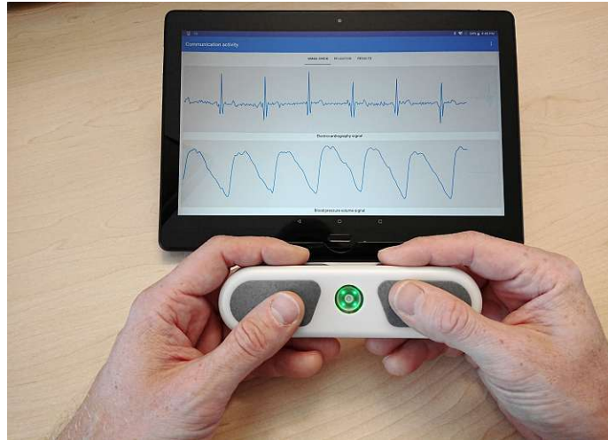
Figure 3.9: The smartPWA as seen during measurement. It is held with both thumbs on the conductive surfaces and the right index finger on the PPG sensor. The signals are immediately processed and visualised on the connected tablet.
