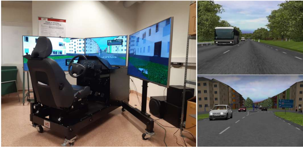
Figure 3.8: Left: One of the two identical driving simulators used in the pilot trial. Right: Two examples of the simulated driving environment in rural (top) and urban (bottom) surroundings.
