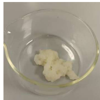
Figure 83: Polymer 22. After the polymer is placed in DMF, it increases in size and becomes soft and malleable.
