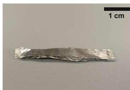
Figure 91: After the polymer has swollen, the test strip is removed from the mold and any excess aluminum foil is cut off.
