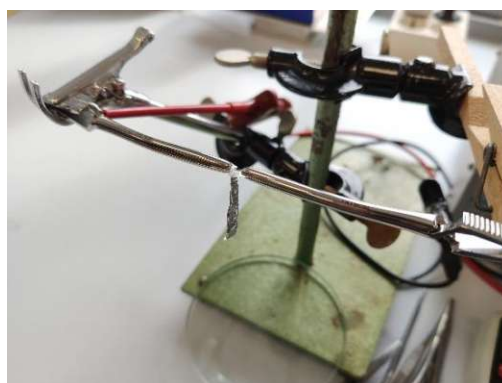
Figure 92: The test strip was fixed by two aluminum clamps and a voltage between 5-20 V was applied.
