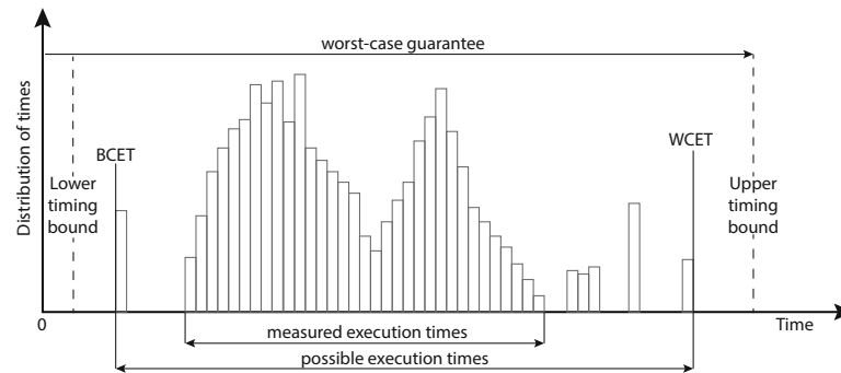
Figure 9.1: Basic notions of timing analysis [WEE + 08].
