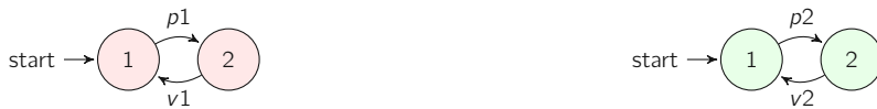
Figure 8.17: The two semaphores S_1 and S_2 for synchronising the two processes A and B .
