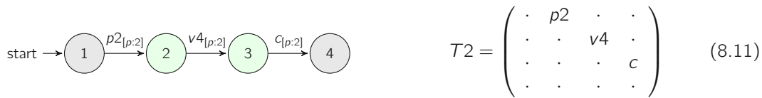
Figure 8.27: Process T2 adjusted with all semaphores and with priority 2.
