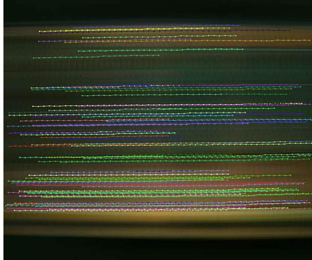
Figure 5.7: Synthetic image with found feature tracks longer than 20 subsequent images. Ideally, feature tracks appear straight with uniform spacing between single feature points.
