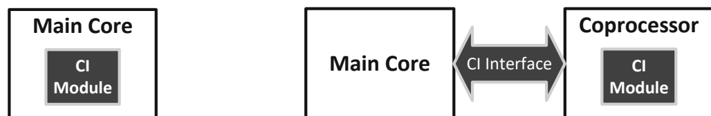
(a) In-pipeline integration [28]: CI hardware added inside the main core as a separate execution unit. (b) Interface-based integration : CI hardware integrated with a CI interface and an external coprocessor.
