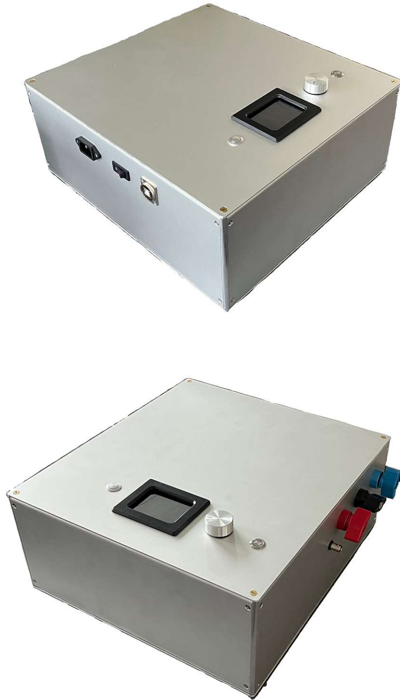
Figure 1.1: Completely assembled pulse generator
