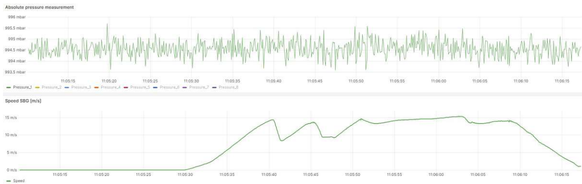
Figure 3.6 – Speed and total pressure of channel 1 during rake validation
