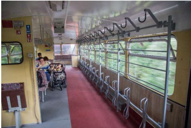
Figure 46: Interior of 5095 railcar rebuilt for bike transport on the Murtalbahn. Author photo
