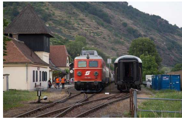
Shunting of summer solstice special trains. Sharp turnout for track nearest to station can only be used at low speeds.
