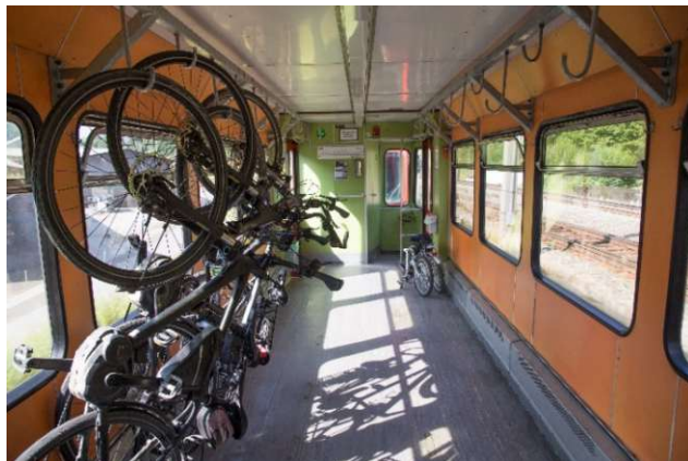
Figure 47: Interior of Hungarian BzMot railcar equipped for bicycle carriage. Author photo.
