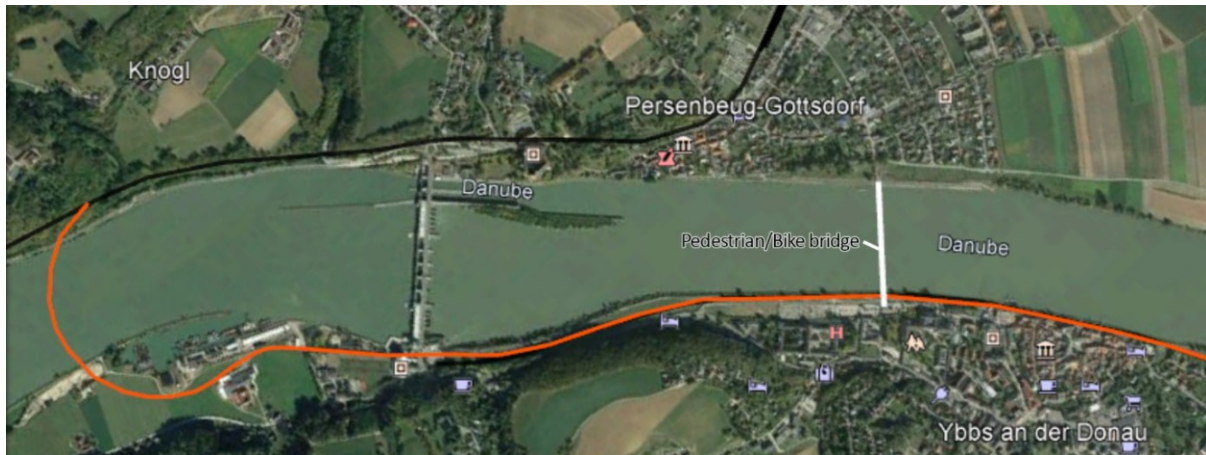
Figure 64: Potential alignment for a direct rail connection to Ybbs and bridge for non-motorized transport Source: Author drawing, Google Earth
