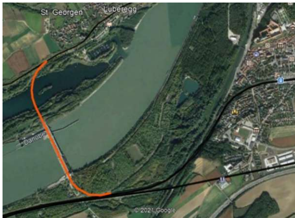
Figure 57: Potential alignment of railway connection Melk-Donauuferbahn
