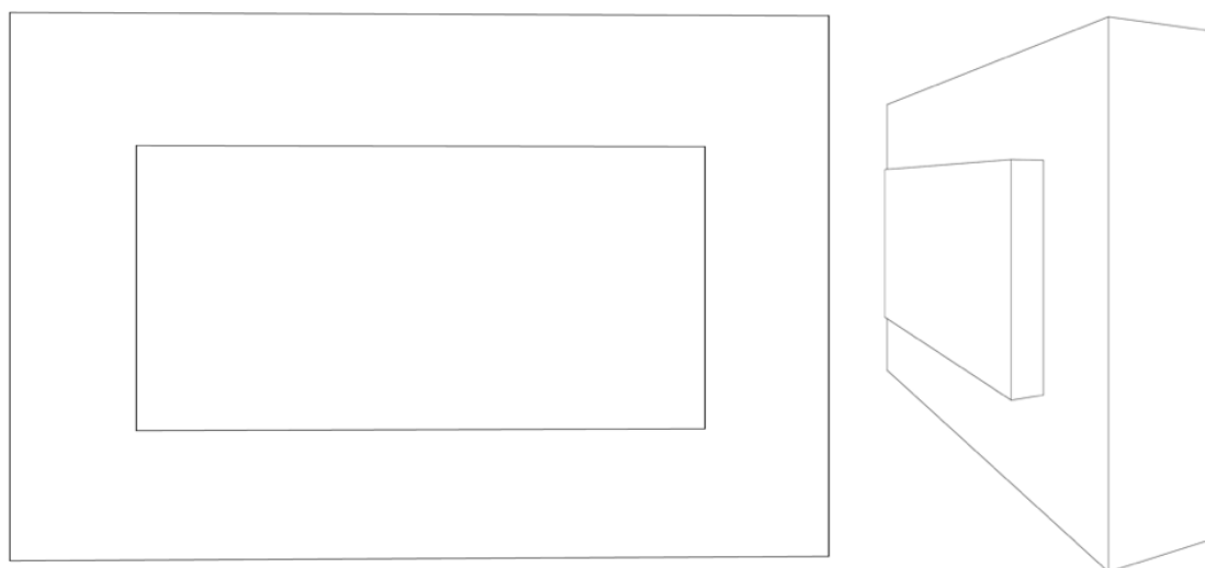
Figure 4 Schematic views of the ashlar with drafted margins; frontal view (left) perspective view (right)
