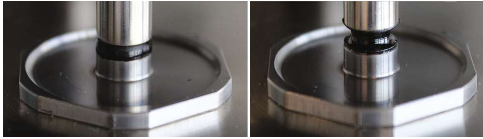
Fig. 1 Cylindric specimen shape (left) and hyperbolic specimen shape (right)
