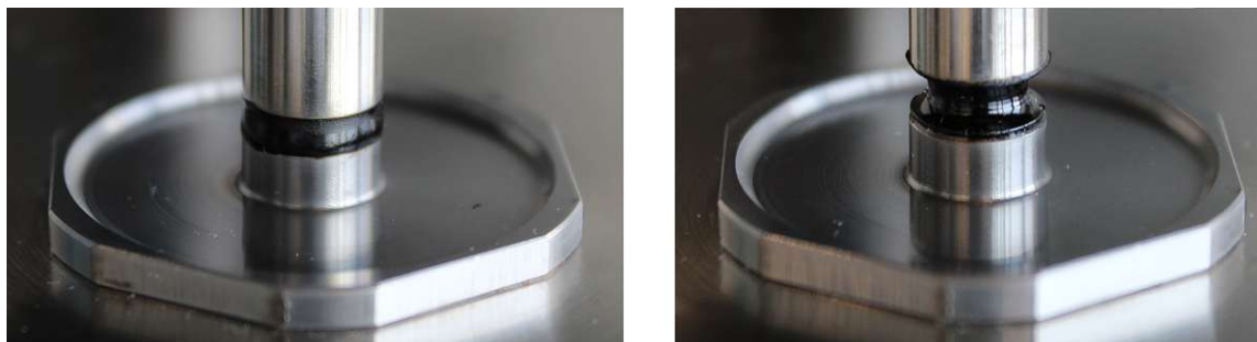
Fig. 2.5: Cylindrical (left) and hyperbolic (right) specimens
