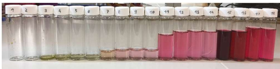
Fig. 2. All 18 fractions of the dynamic streamlined extraction. Fractions 1–2 (1 vol% EtOH), Fractions 3–6 (10 vol% EtOH), Fractions 7–10 (20 vol% EtOH), Fractions 11–14 (50 vol% EtOH) and Fractions 15–18 (acidified EtOH).
