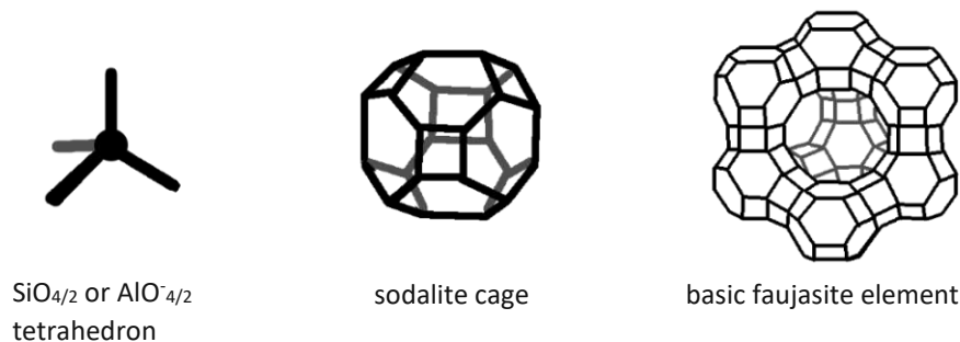
figure 18: Different levels of zeolite structure
