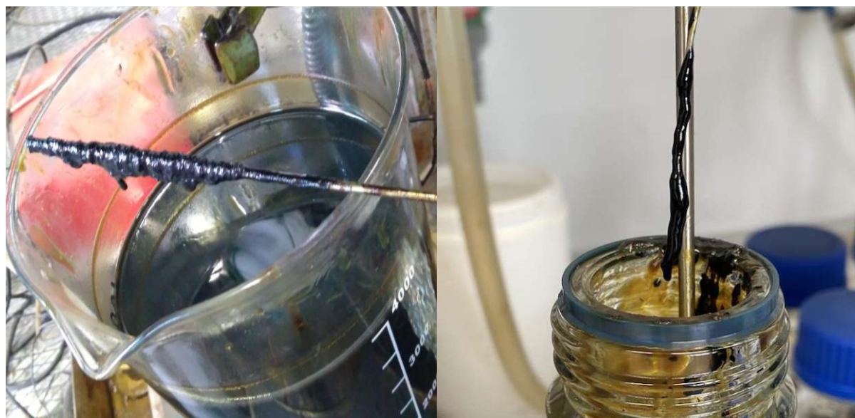
figure 22: Pictures of the solids formed when SDPOcw, SDPOsun respectively are mixed with VGO (admixture 10 %). Left: thermometer that was in 4000 mL of a 10 % admixture SDPOcw; Right: wire that was in 100 mL of a 10 % admixture SDPOsun
