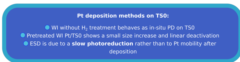
Figure 6.21: Summarized observations concerning the Pt deposition methods on TS0. It was found that the reduction in a pretreatment still leads to some size increase and a small deactivation, and that the main reason for the ESD is the size increase due to a slow photoreduction in samples where Pt is reduced by illumination.
