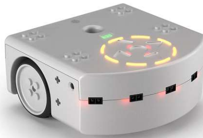
Figure 2.2: The educational robotics equipment Thymio is a small mobile robot with the dimensions approximately 15 cm wide, 12 cm long and 4 cm high and has three different actions, all based on obstacle detection by the infrared sensors and presented as moods such friendly, curious and shy. A series of LEDs and sound effects enhance those moods. The robot is gender-neutral and in a mantle of a white box also as a playground to added the construction with possible lego brix. The robot is useful for workshops for all young students.
