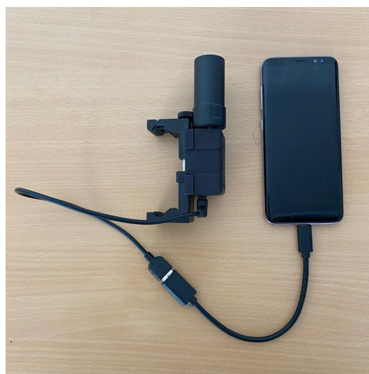
Fig. 1 The REDCatch Smartphone RTK device (on the left) connected through USB to an Android Samsung S8 smartphone (on the right)
