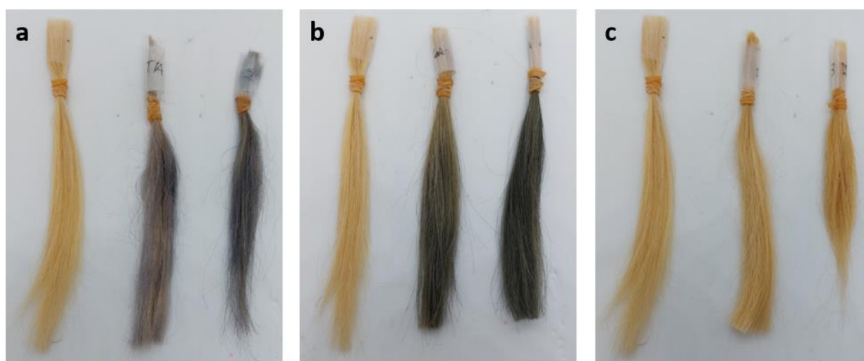
Figure 37: Dyed hair samples. a) TA-Fe, b) CaAc-Fe and c) LS-Fe dyed hair. In each picture the left hair strand is undyed, the middle one is dyed once and the right one was dyed 3 times.
