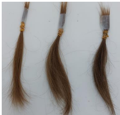
Figure 38: Dyed hair sample with unbleached hair dyed with caffeic acid -Fe. The left strand is undyed, the middle strand was dyed once and the right one was dyed 3 times
