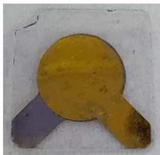
Figure 13: QCM crystal consecutively dipped into paracoumaryl alcohol and iron solution with blue spots on the surface.
