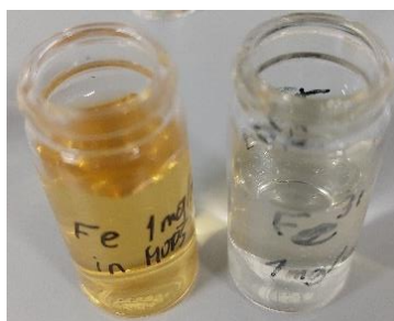
Figure 11: 1 g/l of \text{FeCl}_3 \cdot 6\text{H}_2\text{O} dissolved in 10 mmol/l MOPS and water for comparison.
