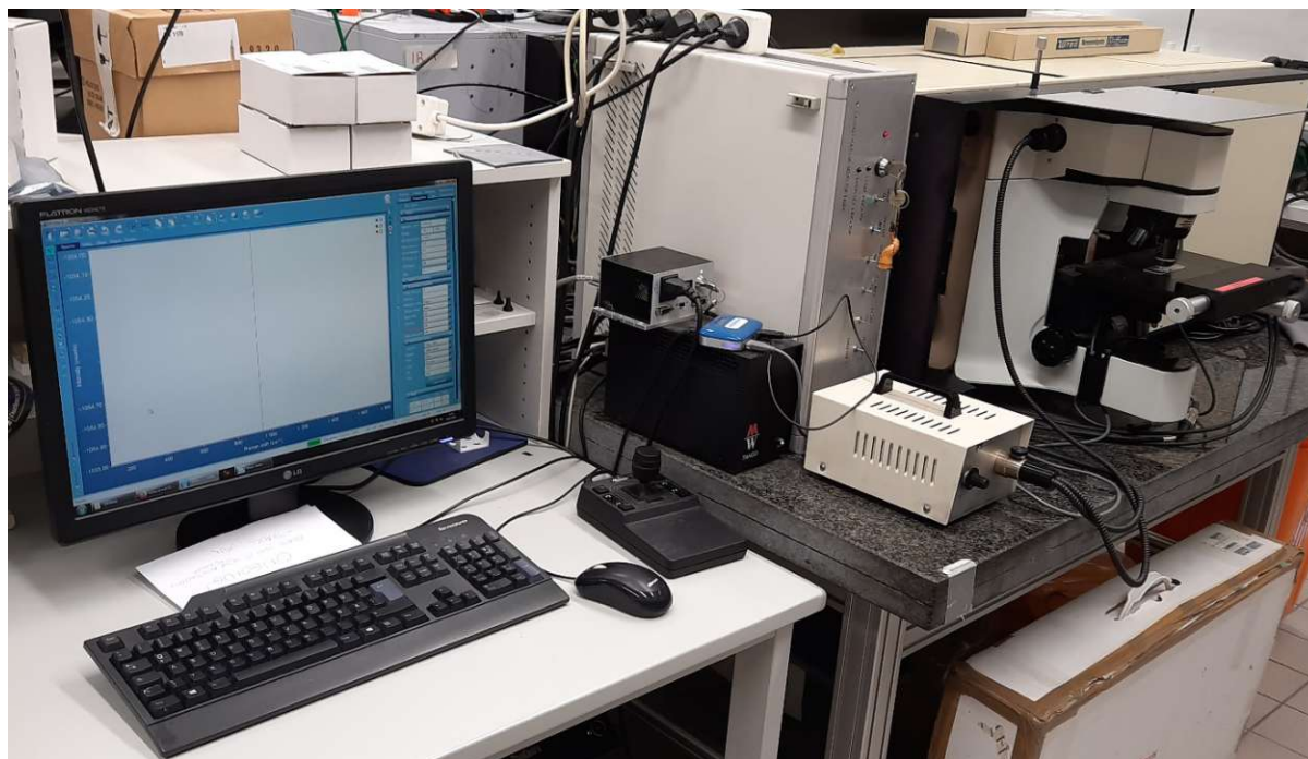
Figure 3.10: HORIBA LabRAM 800 HR dispersive Raman microscope (facility at Institute of Chemical Technologies and Analytics (research group of process analytics), TU Wien, Vienna) utilized for the Raman spectroscopic studies on all the samples investigated in this thesis.
