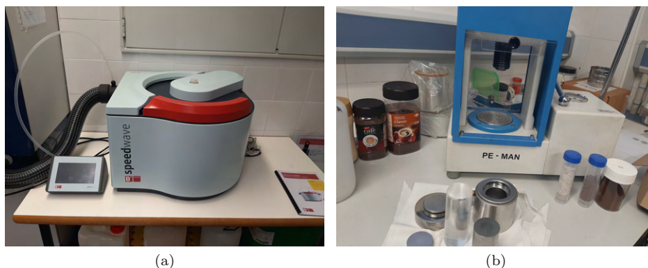
Figure 24: (a) Speedwave XPERT microwave system and (b) PE-MAN manual hydraulic press with pellet preparation equipment.
