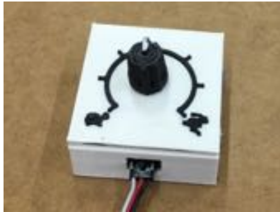
Figure 12.14: 3D-printed case and knob for potentiometer.
