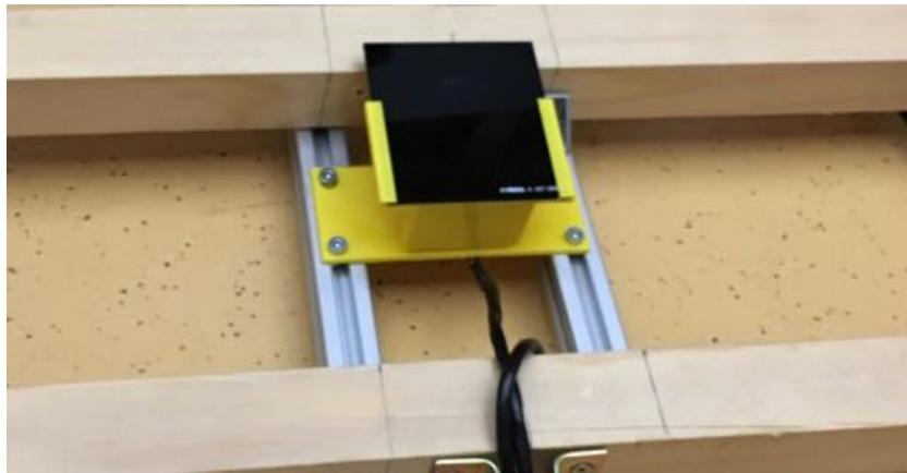
Figure 12.6: Mounted camera with infrared passing filter on top.
