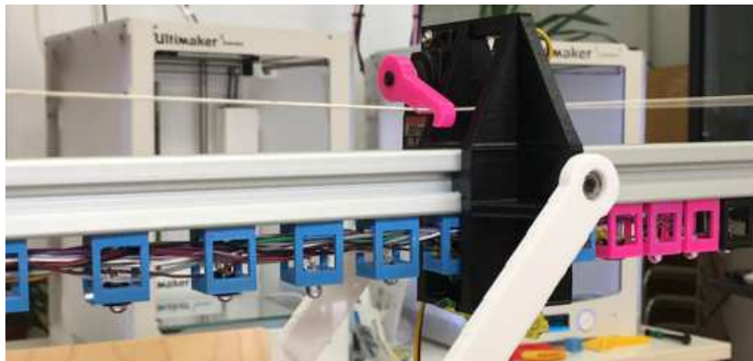
Figure 8.10: Infrared LED feedback positioning system and servo motor replacing the pull solenoid.
