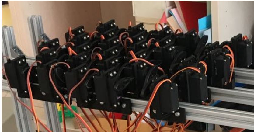
Figure 10.2: Third iteration: One servo per fret approach, servo horn extension.
