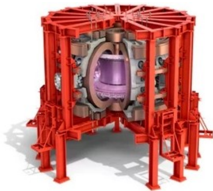
Figure 1.6: Diagram of ASDEX Upgrade with its supporting structure (red), main field coils (bronze), vacuum vessel (silver) and plasma (purple). Adapted from [15].
