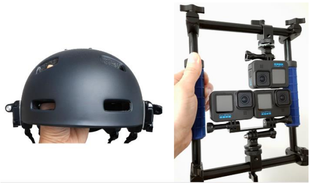
Figure 5. The POC Crane Mips helmet onto which the three cameras can be mounted (left); Three GoPro cameras mounted inside a frame composed of standard camera rig components (right).
