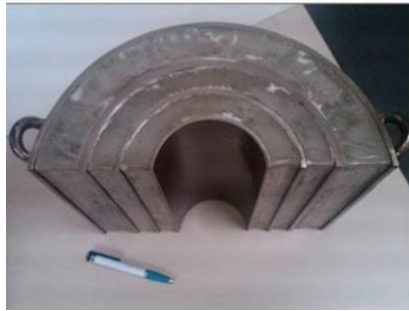
Figure 18 Demonstration of the several sections of cemented casings in the well
