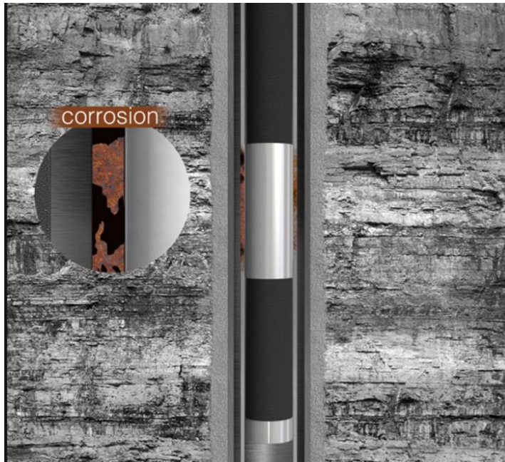
Figure 24 Casing Patch (against corroded area or pipe) Source: (Saltel Industries, 2020)
