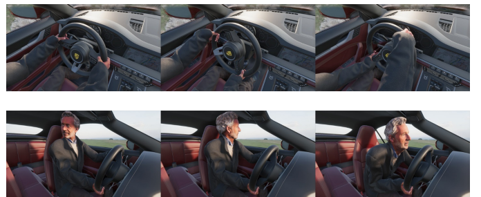
Fig. 3: Illustrations of possible applications of the procedural animation workflow based on inverse kinematics. First row: Grabbing different objects in the vehicle interior such as the steering wheel. Second row: Variation of poses in the vehicle interior.
