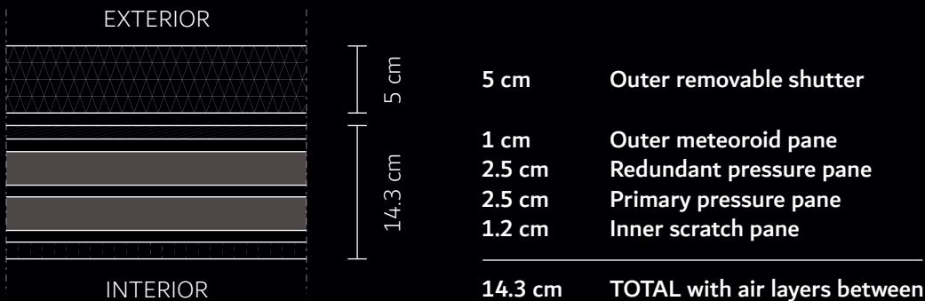
Fig. 4.13 | X-plor Wall and Window Glass sections
