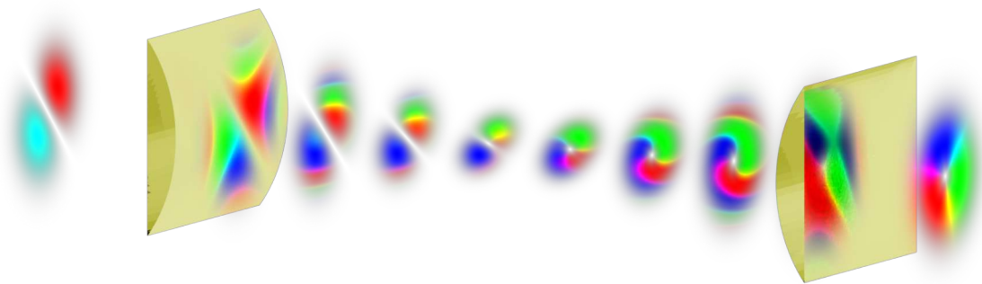
Figure 3.: Schematic principle of the mode converter. A HG beam rotated by 45^\circ (left) enters a lens system comprised of a pair of cylindrical lenses (which can be realized in the TEM as a combination of a round lens and a quadrupole). One component goes through the focus, resulting in a phase shift that can be tuned to produce an LG EVB (right).
