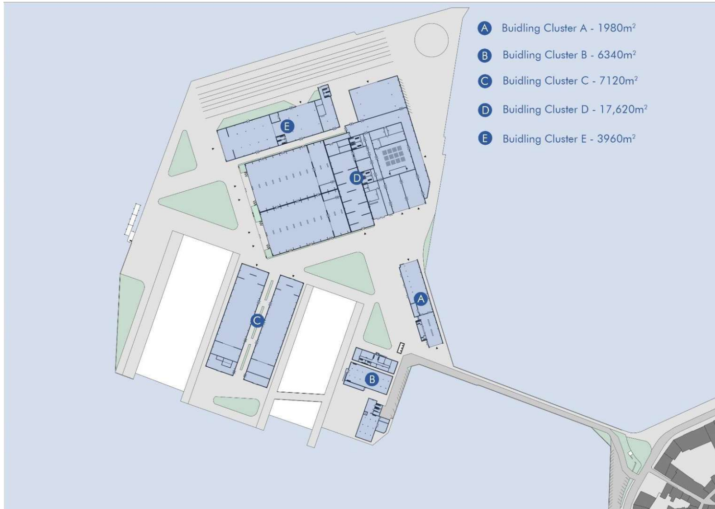
Figure 77 | Ground floor plan of a categorisation of buildings on site into clusters with represented usable interior space
