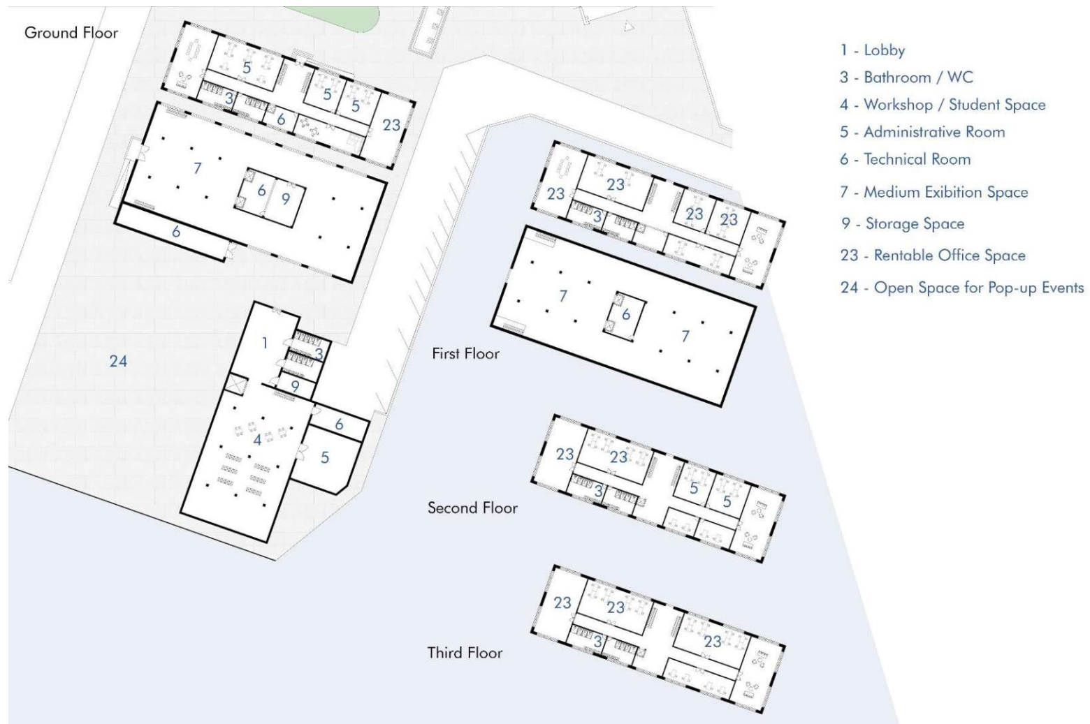
Figure 82 | Floor plan of Cluster "B"; With detailed program layout of interior space
