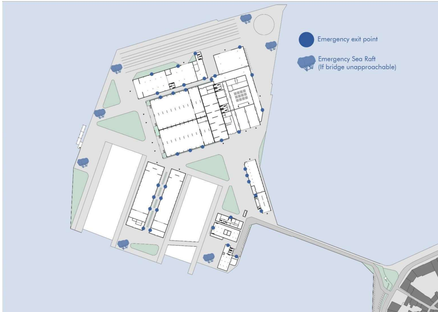
Figure 76 | Ground floor plan with represented emergency exit points from of the buildings and the emergency sea raft locations in case the bridge would ever become inaccessible
