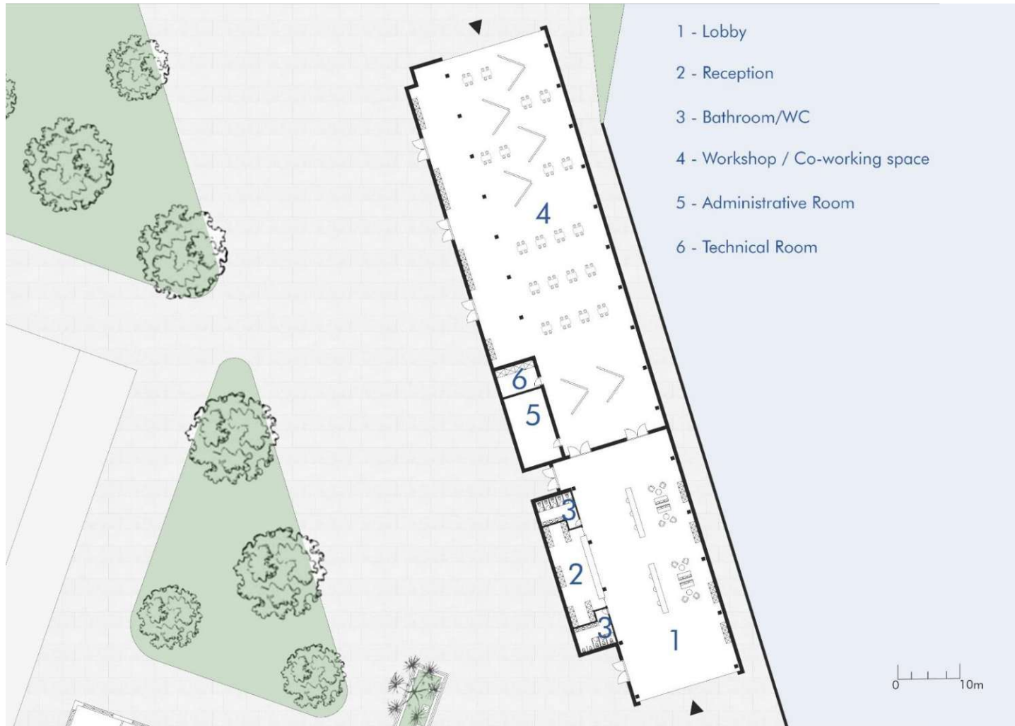
Figure 79 | Floor plan of Cluster "A"; With detailed program layout of interior space
