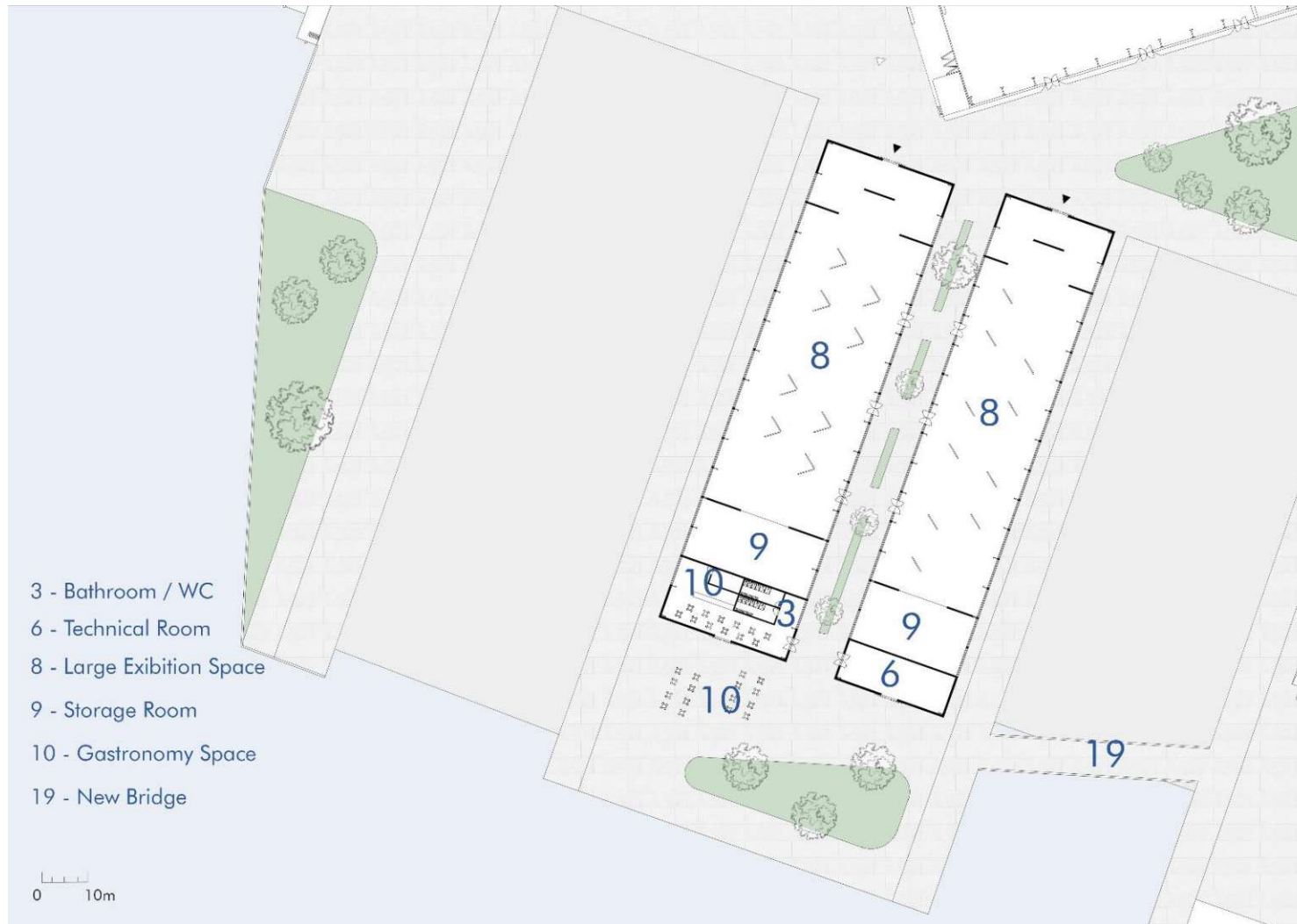
Figure 85 | Floor plan of Cluster "C"; With detailed program layout of interior and exterior space
