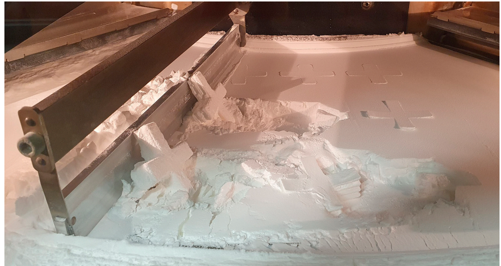
Figure 2. Part shifting leads to total process abortion at the PBF-LB/P system used in this study. Components were completely torn out of the powder bed via the coater blade. The inside of the machine must be completely cooled and cleaned before the entire job can be restarted.
