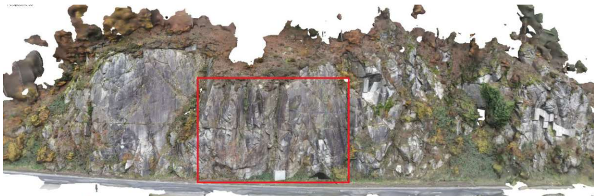
203 204 Figure 5: 3D photogrammetry model (Agisoft, 2021) of the Tiefenbach rock face. The structural geological analysis was 205 limited to the marked area (Red).
