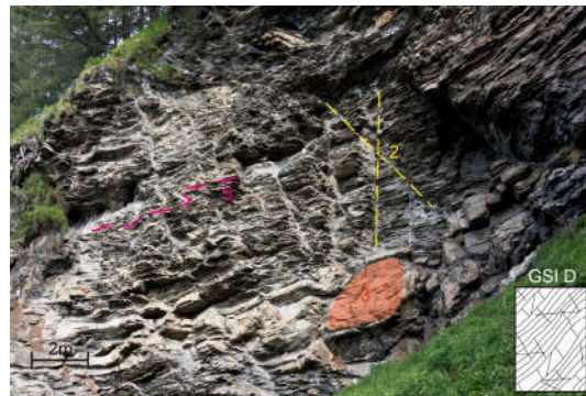
Figure 4. Outcrop, representative for strongly folded and jointed rock mass of Bündner Schists in the valley of Vals: S—schistosity (magenta), 2—conjugate discontinuities (yellow), 3—fault plane (red).
