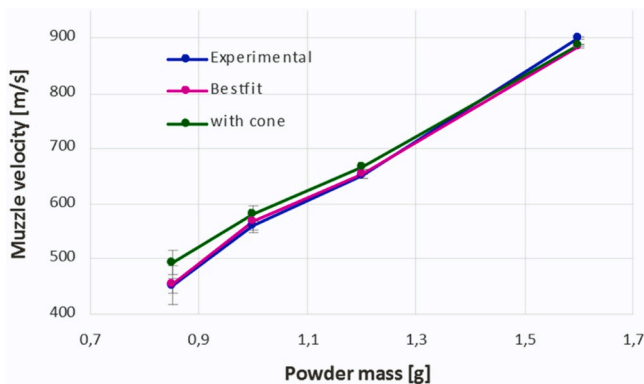
Fig. 15. The experimentally measured v_0 values compared to the calculated v_0 values with the discussed velocity-dependent friction model as a function of the four investigated powder masses. The error bars correspond to the standard deviations of the muzzle velocities.
